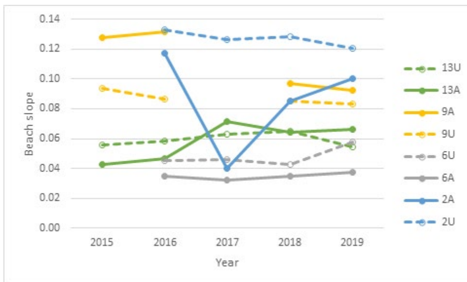
Figure B23. Average beach slope (m) measured at each North site pair in Snohomish County, WA; where solid lines represent armored locations and dashed lines represent unarmored locations. Beach nourishment occurred between survey years 2016 and 2017.
