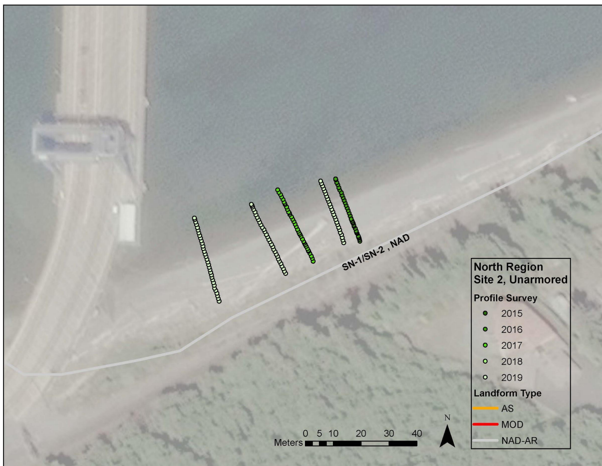
Figure B5. Location of profile survey points, by survey year, collected with Trimble RTK GPS. At least one profile was collected at center of 50-m sample transect each survey year.
