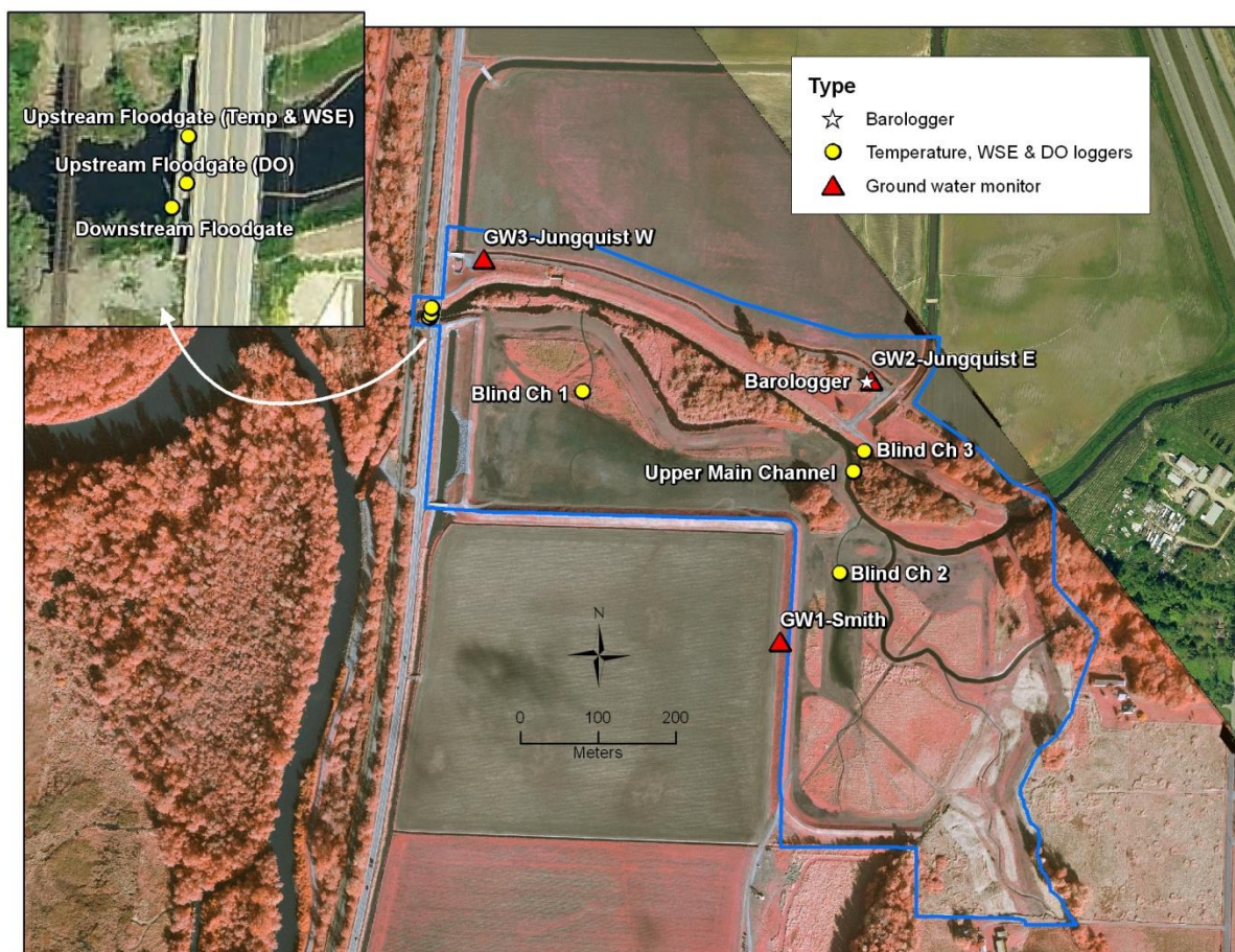
Figure 1-3. Location of barometric pressure (barologger), groundwater, water surface (WSE), and DO monitoring equipment for Fisher Slough project site. Datalogger at Downstream Floodgate also includes floodgate-door-openness monitoring. Project area is outlined in blue.
