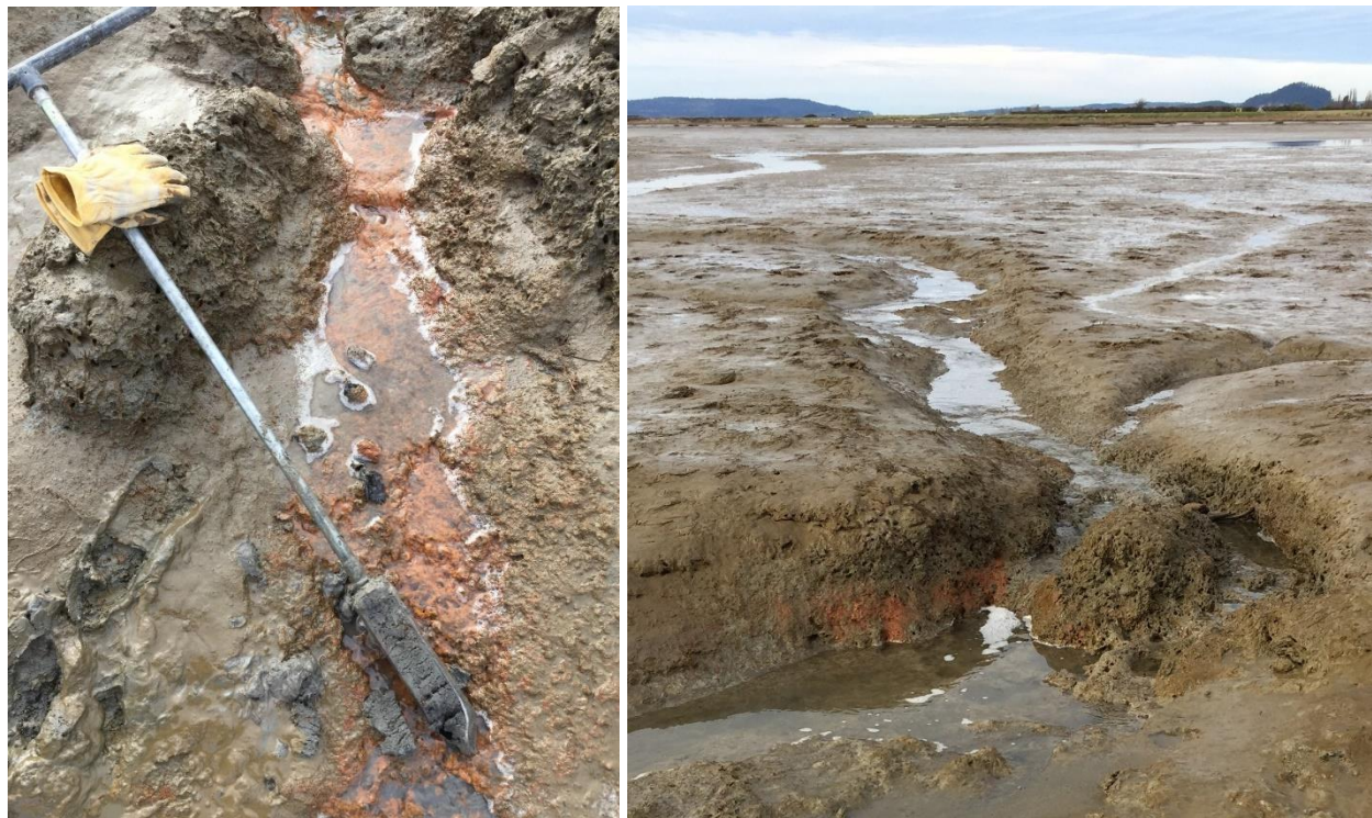
Figure 12. Surface exposure of clay soils in shallow tidal channels showing rusty colors diagnostic of iron-oxides bound to clay particles. Sediment in the auger is not rusty because at depth it is not exposed to oxidation. These tidally-eroded channels have limited depth due to the erosion resistance of the clay.
