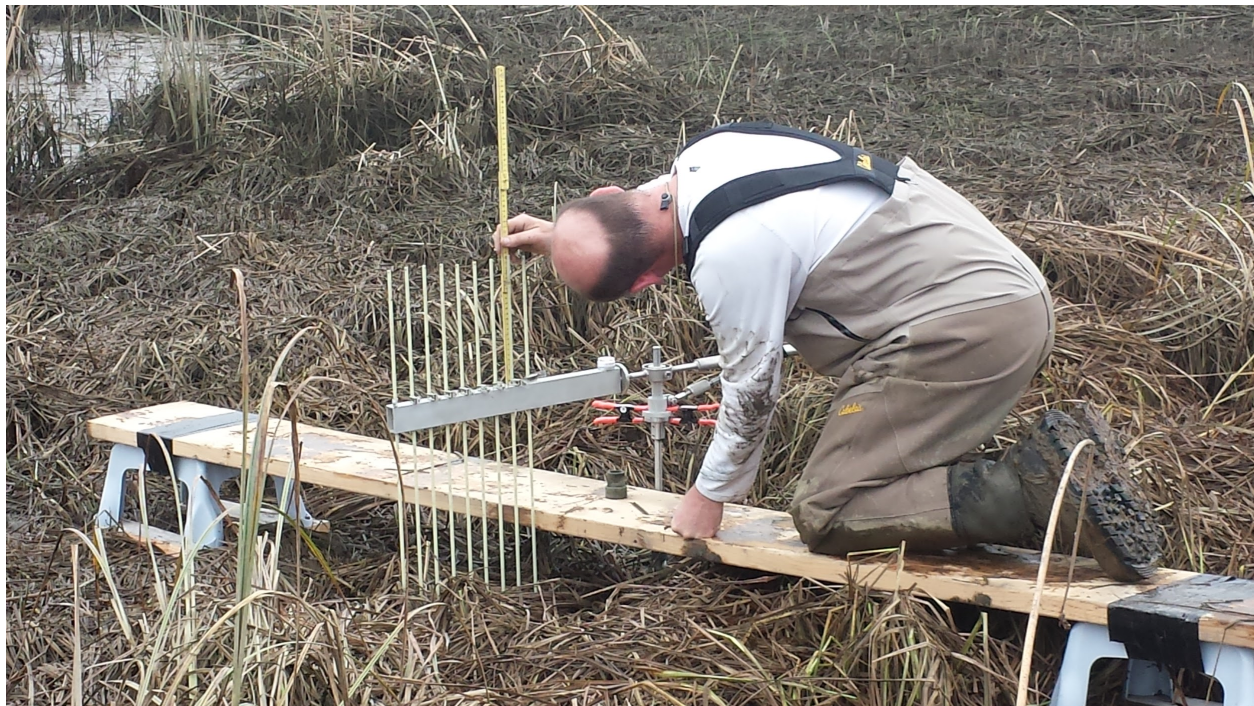
Figure 13. Reading RSETs in a reference marsh. A platform is used to prevent footprints from changing surface elevations within the monitoring site.
