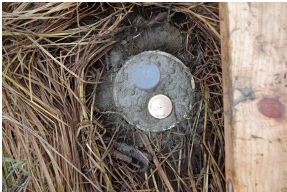
Figure 12. RSET rod cap and datum secured at surface with concrete.
