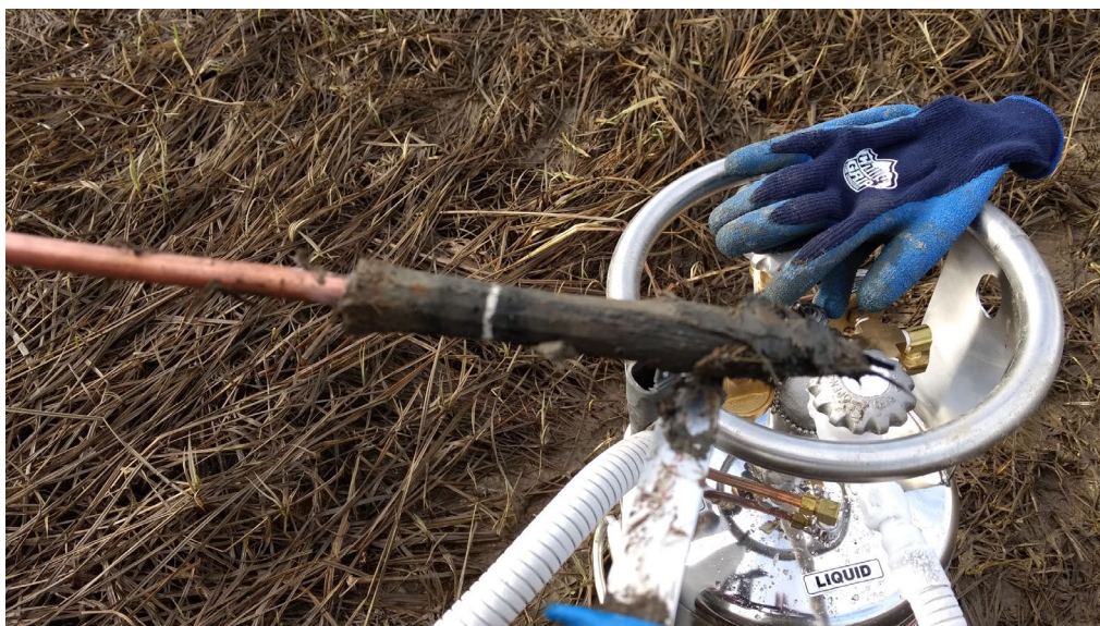
Figure 15. A sediment core taken with the cryocorer. The white line of the feldspar MH is visible on the core that is frozen to the probe. The distance from the surface to the top of the MH is measured on all four axis of the core.
