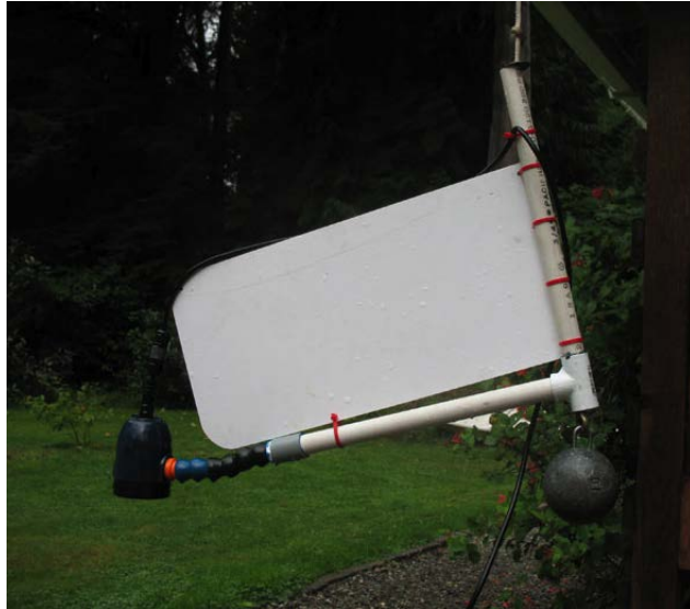
Figure 10. Drop camera apparatus used in sampling for fish and mobile invertebrates
