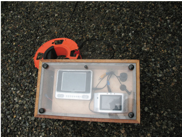
Figure 11. Monitor and recording equipment contained in weatherproof housing.
