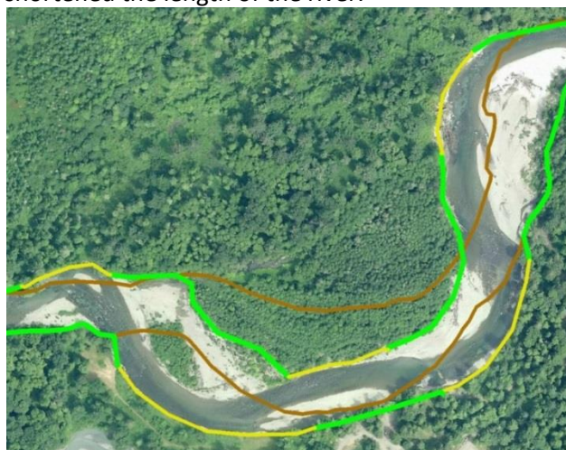
Figure 5: Example of 2002 river bank alignment (brown lines) versus 2011 alignment (yellow/ green lines). 2011 river banks are coded as natural/stable (green) and natural/unstable (yellow).
