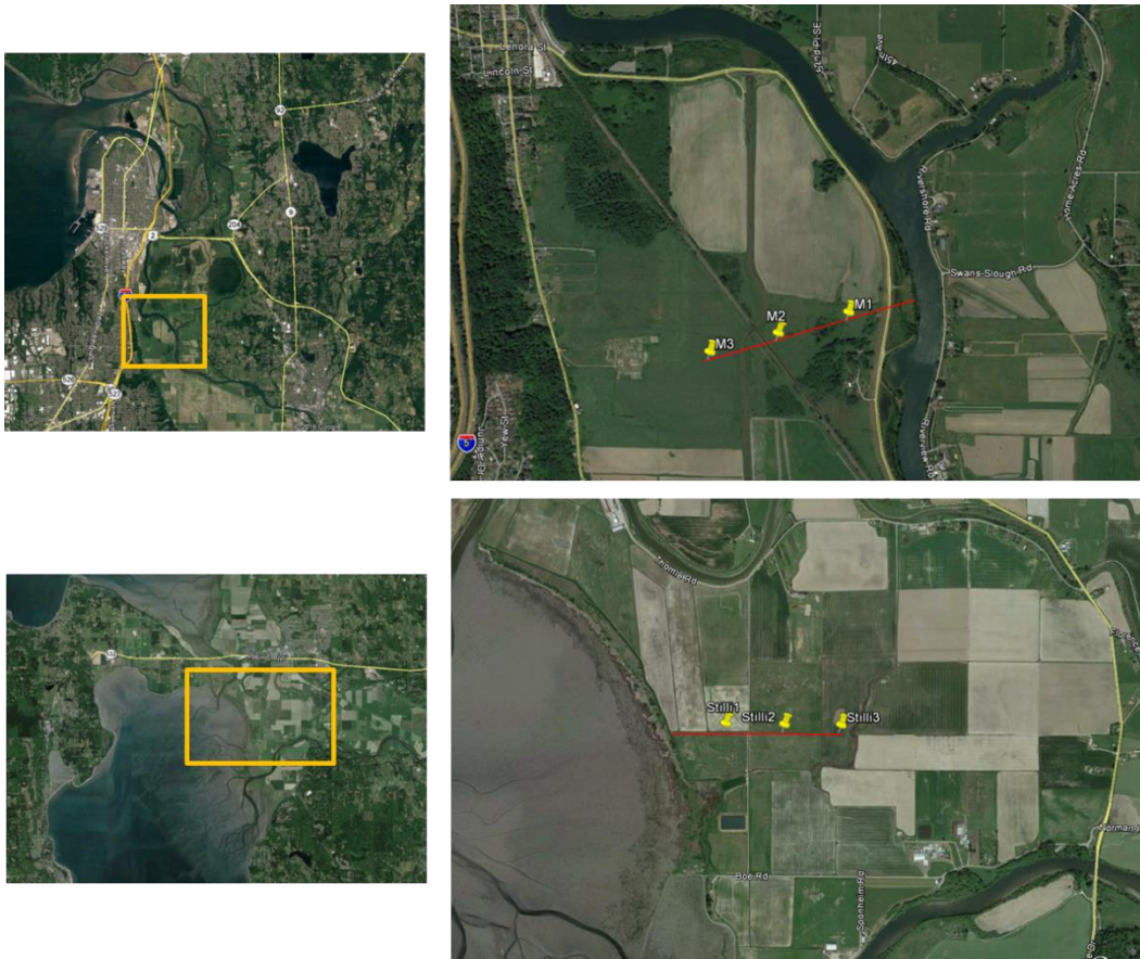
Figure 1. Maps showing groundwater monitoring array in the Marshlands of Snohomish Estuary (top) and Stillaguamish river-delta (bottom). Surface water monitoring sites will be sited in nearby estuary channels or nearshore along with barometer to develop the time-series forcing on groundwater levels observed in monitoring wells.
