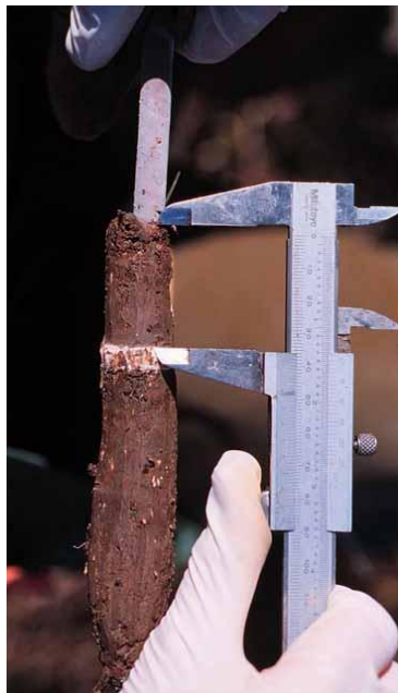
Figure 14: Free-core sample showing accretion above artificial horizon. (Image from USGS Surface Elevation Table website, Cahoon and Lynch).
