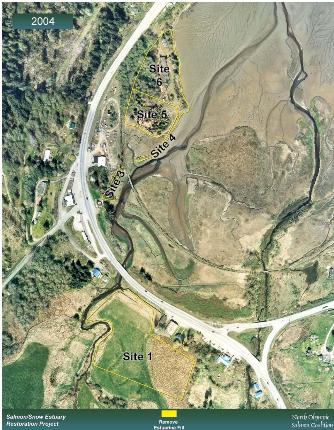
Figure: 2004 aerial shows project area prior to fill removal and tidal channel construction.
