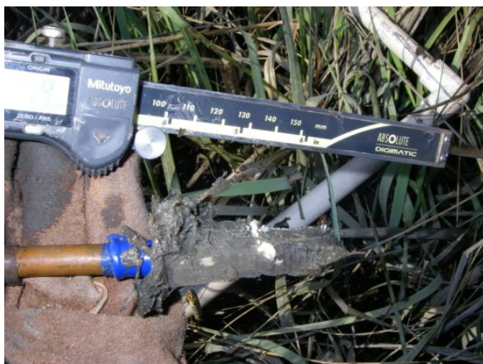
Figure 22: Example of cryo-core that needed scraping to expose the feldspar
