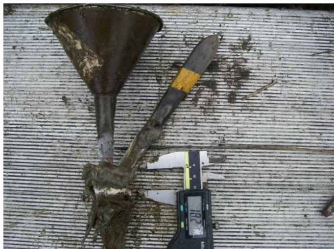
Figure 21: Example of good feldspar layer; note the digital calipers and metal scraper/spatula.
