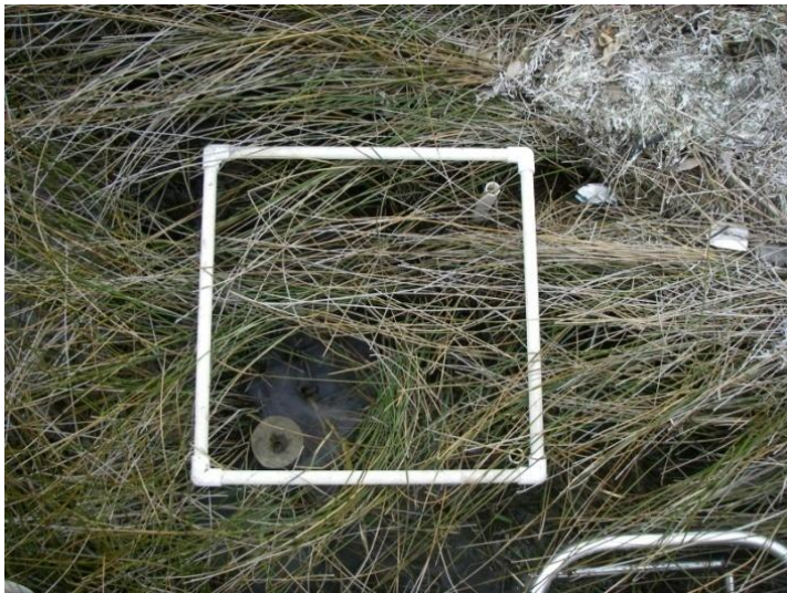
Figure 19: Example of sampling a Marker Horizon plot; note the PVC poles, \frac{1}{4} meter quadrat and cryo-core funnel
