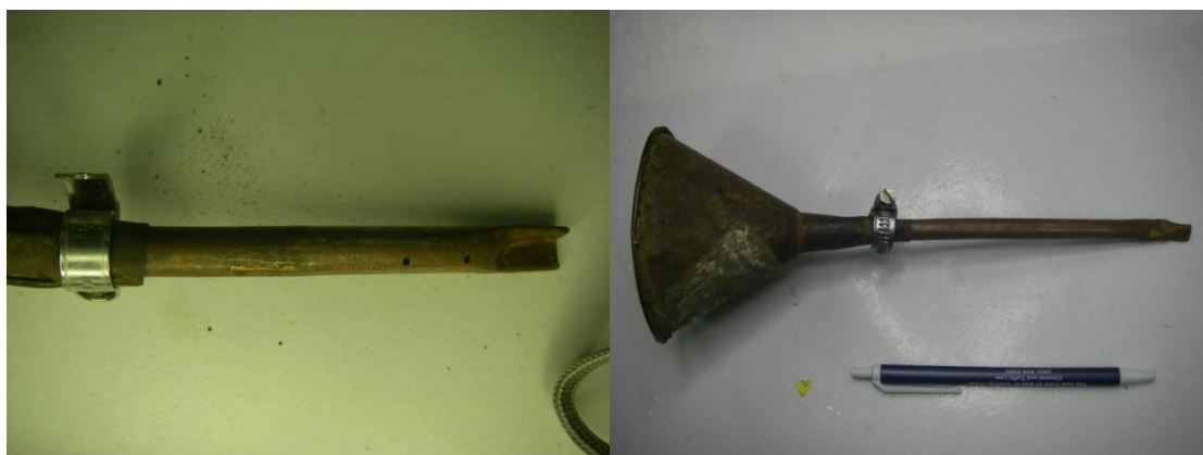
Figure 20: Cryo-corer: Note the crimped end of the copper tubing, staggered holes drilled to help freeze the deeper sediments, and the hose clamp attaching the funnel securely to the copper tube.
