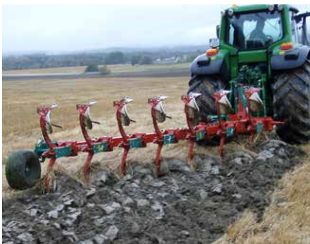
Figure 9.6. Moldboard plowing may be required for adequate field preparation, especially under organic management. PHOTO BY ÅSMUND LANGELAND, LICENSED UNDER CREATIVE COMMONS SA 3.0. WIKIMEDIA COMMONS.
