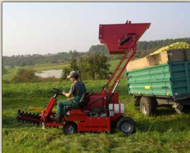
Figure 5.8. Mid-sized units like this OB 80R can be equipped with an unloading hopper. PHOTO COURTESY OF PRODUCETECH.
