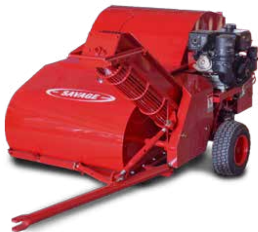
Figure 3.11. The Savage model 8042 pecan harvester is self-powered and can be towed behind an ATV or lawn tractor. PHOTO COURTESY OF SAVAGE EQUIPMENT.
