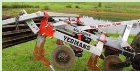
Figure 2.13. A Yeomans Keyline plow. PHOTO BY MILKWOOD. NET, LICENSED UNDER CC BY-NC-SA 2.0.
