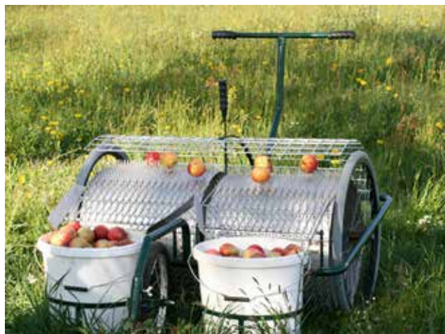
Figure 3.3. Rolling drum harvesters such as these made by Huemer Obsterntetechnik might be appropriate for smaller cider plantings. Basic models are hand-pushed, with options for adding an electric assist motor. A larger unit can be pushed by a lawn tractor or walk-behind tractor. SOURCE: HTTP://WWW.OBSTSAMMLER.COM/EN/
