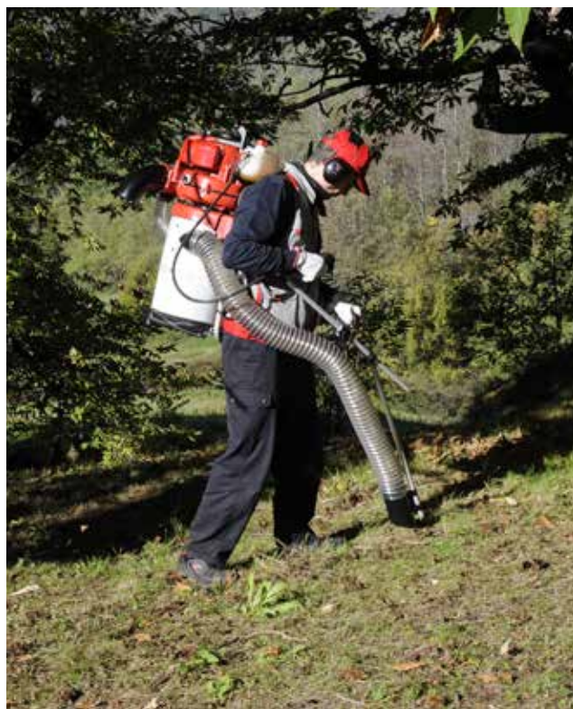
Figure 3.14. A backpack vacuum harvester by the European company Cifarelli. According to the manufacturer, the vacuum is suitable for hazelnuts, chestnuts, acorns, olives, and almonds.
