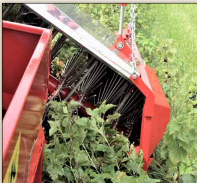
Figure 5.5. The shaking rods inside the harvest unit. PHOTO BY KEVIN WOLZ.
