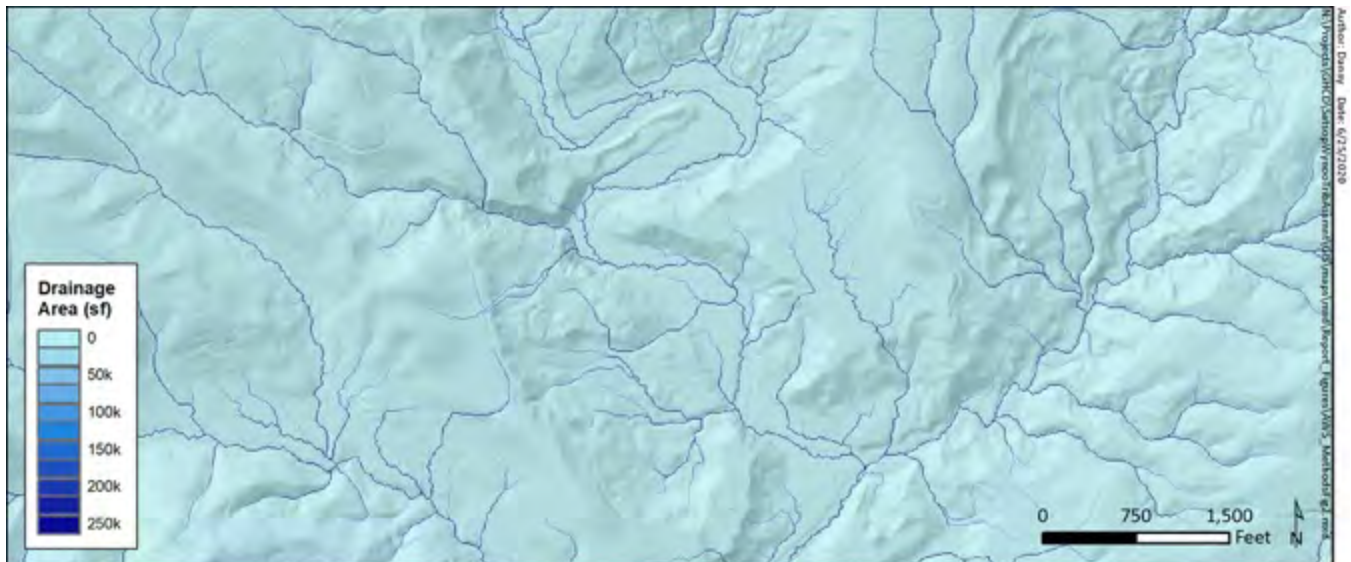
Figure 5. Stream network and associated drainage area derived from flow accumulation analysis on the DEM for the same example location along the Upper West Fork Satsop River illustrated in Figure 4. Note that drainage area is computed for every pixel in the DEM, and pixels with a drainage area greater than 250,000 square feet (sf) (dark blue in the figure) are designated as the stream network.
