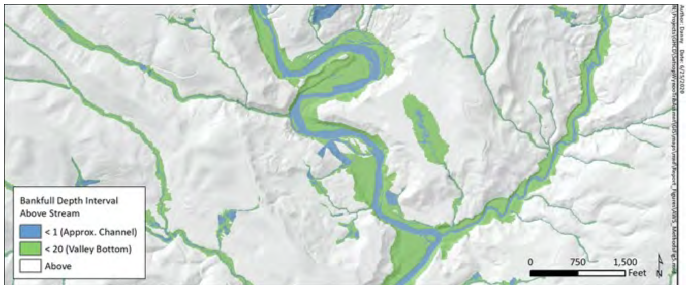
Figure 8. Valley bottom and channel extent polygons derived from the relative elevation raster for each reach for an example location along the Upper West Fork Satsop River.
