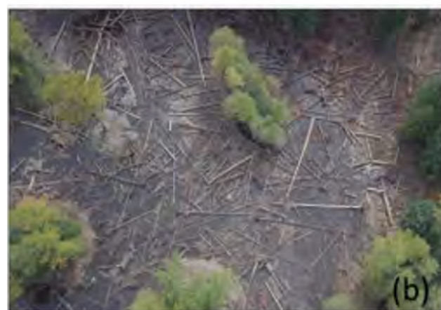
Aerial photographs of (a) pre- and (b) post-treatment with valley reset approach in Staley Creek, eastern Oregon from Figure 8 of Powers et al. (2018). Note single thread channel in (a) as opposed to multiple flow paths and high wood loading in (b).
