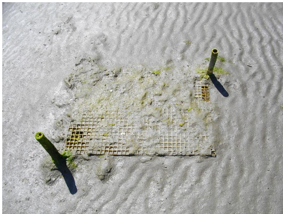
Figure 7. The gridded plastic markers in the bare tidal flat were eroded, exposing the markers and not allowing for the sampling of accretion in that area.
