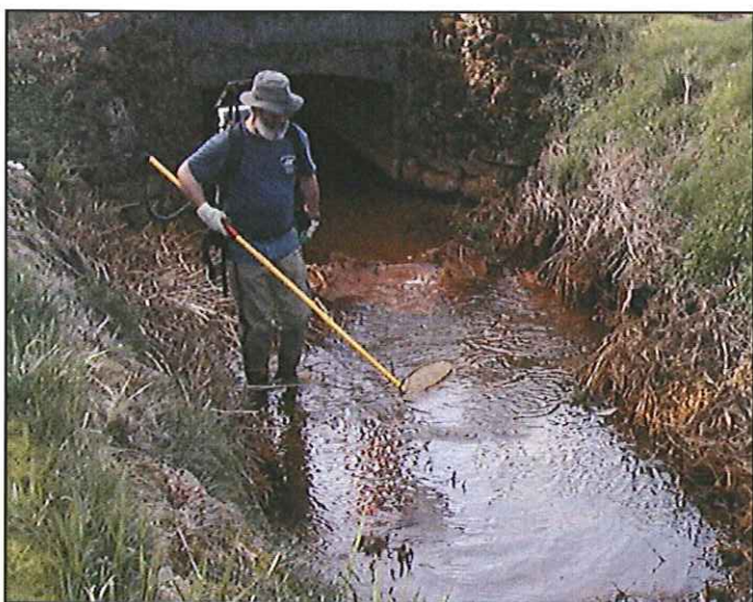
Electrofishing with a Backpack Shocking Device
