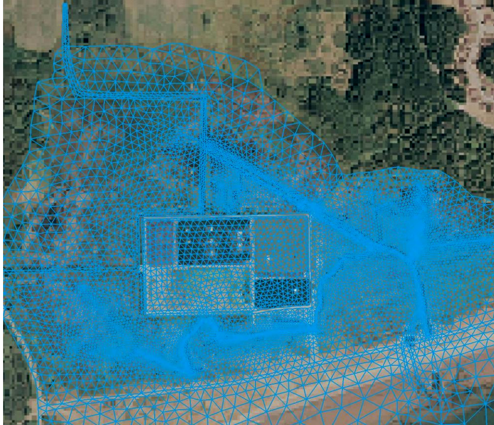
Figure 2. Battelle/PNNL FVCOM hydrodynamic model grid for the Crescent Harbor Restoration site. An accurate estimate of freshwater inputs to the system is essential for obtaining good modeling results.
